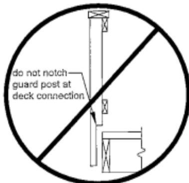
FIGURE 28: NOTCHING AT GUARD POSTS
